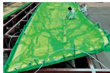
The infusion process improves the strength of the composite and offers superior mechanical properties to the traditional process.
