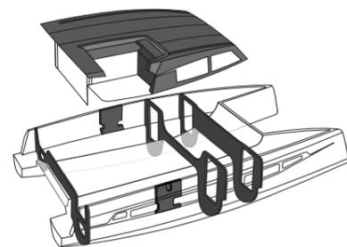
The OC is equipped with a large number of laminated carbon elements as standard: The entire structure, the entire roof and the daggerboard reinforcements.
